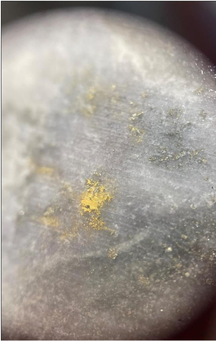
VISIBLE GOLD from drillhole EL-23-08 @ 146.85 m depth. 75.20 g/t Au over 0.50 m
