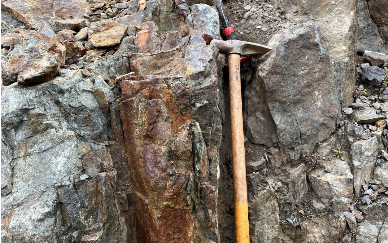
Photo 2: Grab Sample A0519498 from freshly exposed massive-sulphide veining hosting semi-massive pyrite, sphalerite, and minor malachite that yielded 11.30 g/t gold , 89.02 g/t silver, 0.82 % copper, and 1.37 % zinc.
